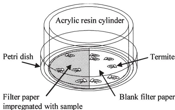
**Fig. 1.** Repellent activity test equipment against *Coptotermes formosanus* composed of two semicircular filter papers, a glass Petri dish bottom and an acrylic resin cylinder
